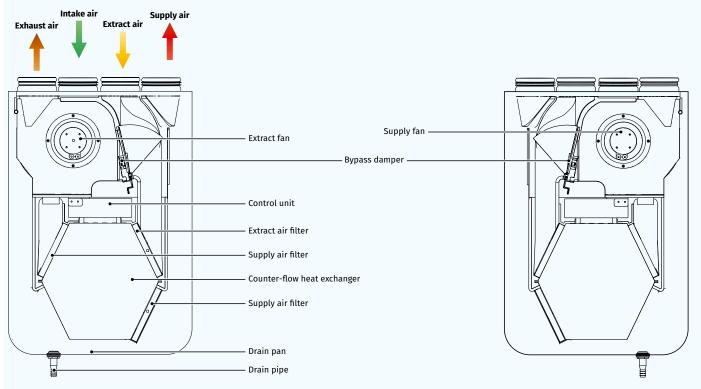
EPP HEAT AND ENERGY RECOVERY AIR HANDLING UNITS
