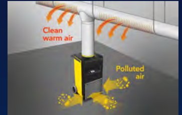
DualHeat blowing-out tower for an even distribution of warm air
