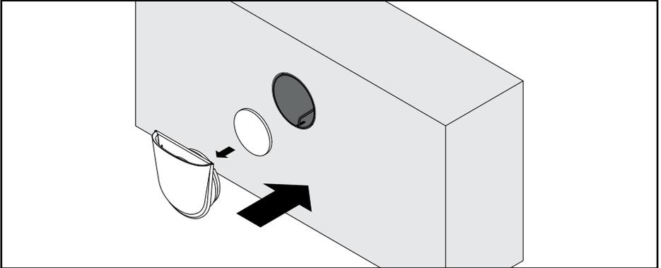
Once all work inside the building has been completed, the inside cover can be installed. Place the filter unit in the slots for the filter inside the cover. Insert the cover into the mounting tube, making sure that the air vent points upwards and that the cover sits tightly.
