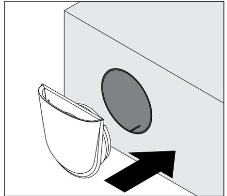
**Step 4:** Carefully reinsert the inside cover into the mounting tube.
