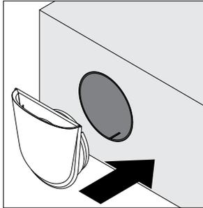
**Step 5:** Reinsert the inside cover (with the air intake pointing upwards) into the mounting tube.
