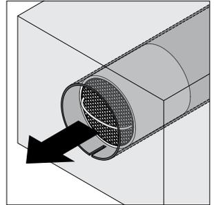
**Step 3:** Pull the heat exchanger unit out of the mounting tube using the strap (2), taking care that the power / control cable is not damaged.
