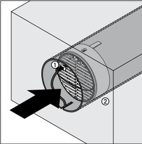
**Step 4 :** Reinsert the cleaned fan unit into the mounting tube. Pay attention to the power cable. Plug in the fan (1). Push the fan unit down into the mounting tube until the spacers touch the heat exchanger (2).
