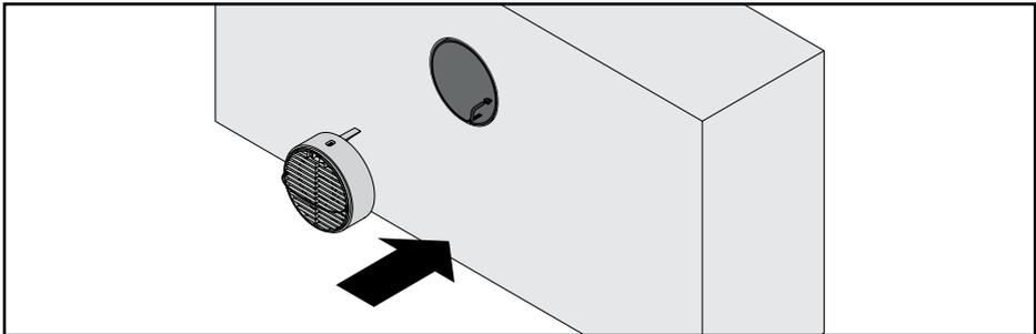
Once the heat exchanger has been installed, the fan unit is then inserted. Set the DIP switches on the fan unit for the desired zone and initial fan direction (see Electrical installation). Mark the settings of the switch on the corresponding sticker.
