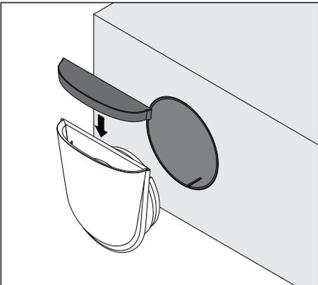
**Step 3:** Place the cap over the air intake. Make sure that the cap fits tightly and completely closes the air intake.
