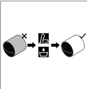
**Step 4:** Clean the heat exchanger unit using a vacuum cleaner or wash with warm water. Only clean the ceramic parts with water! Let the heat exchanger dry.
