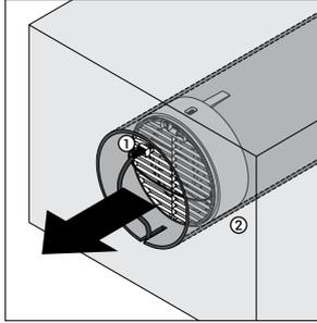
**Step 2:** Unplug the fan (1) Pull the fan unit out of the mounting tube using the strap (2), taking care that the power / control cable is not damaged.
