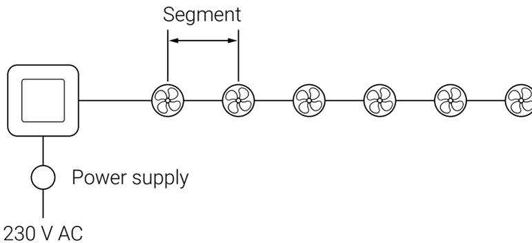
The following table serves as a guide, showing the maximum length per segment (cable length between two units) to ensure adequate supply voltage.
