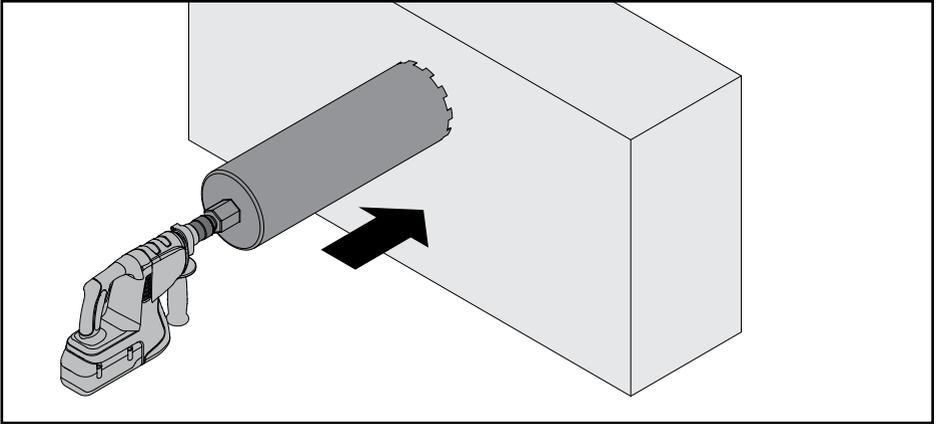
Core-drill a hole in the outside wall using a 162 mm bit. The hole must have a gradient of 1 – 3°, allowing any condensate to flow outwards. It is best to drill the hole from inside to outside.
