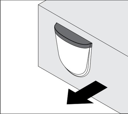
**Step 1:** Pull the inside cover out of the mounting tube.
