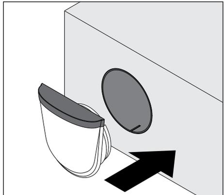
**Step 4:** Re-insert the inside cover into the mounting tube.
