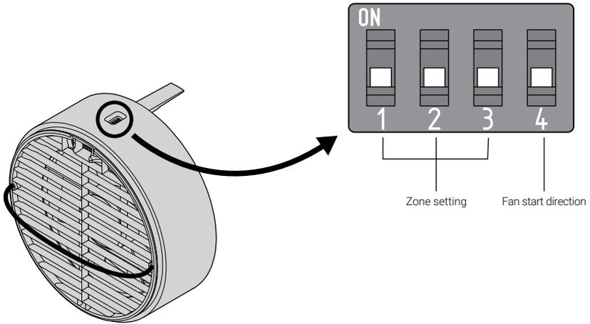
SmartFan fan units are equipped with a DIP switch on the top. During installation, the required zone and initial direction need to be set. Switches 1 - 3 are used to assign a unit to one of the three zones available.
