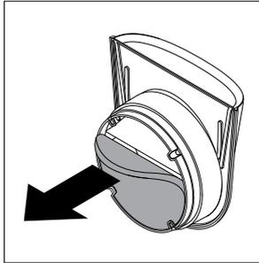
**Step 2:** Remove the filter from its holder.
