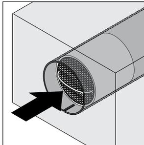
**Step 5:** Reinsert the heat exchanger into the mounting tube, taking care not to damage the cables in the mounting tube.
