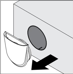
**Step 1:** Pull the inside cover out of the mounting tube.
