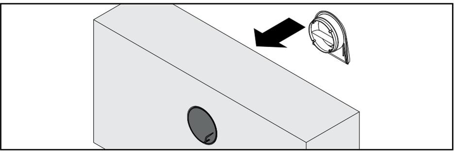
Once all work on the building's facade has been finished, the outside cover can be installed. Remove the plastering cover and insert the outside cover into the mounting tube. Make sure that the outside cover is straight and points downwards (the air vent at the bottom). Due to the special mounting slats, the outside cover can be installed without any tools and sits tight in the mounting tube.
