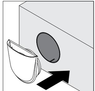
**Step 5:** Reinsert the inside cover (with the air intake pointing upwards) into the mounting tube.
