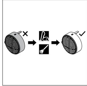
**Step 3:** Using a brush and a vacuum cleaner, clean the fan grille and the rotor blades.
