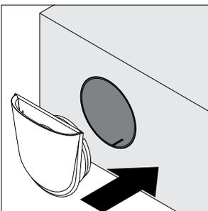
**Step 7:** Reinsert the inner cover into the mounting tube (with the air vent pointing upwards).
