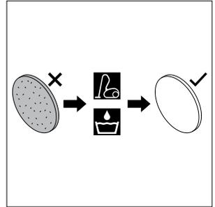
**Step 3:** Check the filter. When necessary, clean or replace it.
