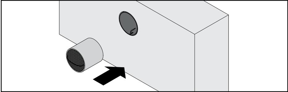
Once all work on the inside wall has been completed and the outside cover installed, the heat exchanger unit can be installed. The exchanger is inserted with the insect filter facing the outside. Push the unit carefully into the mounting tube until it touches the rim of the outside cover.
