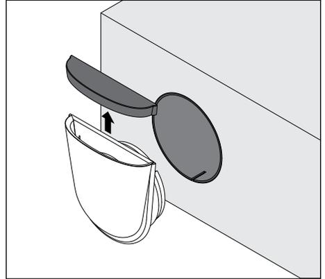
**Step 2:** Remove the cap from the air intake.
