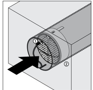
**Step 6:** Reinsert the cleaned fan unit into the mounting tube. Plug in the fan (1). Push the fan unit down into the mounting tube until the spacers touch the heat exchanger (2).
