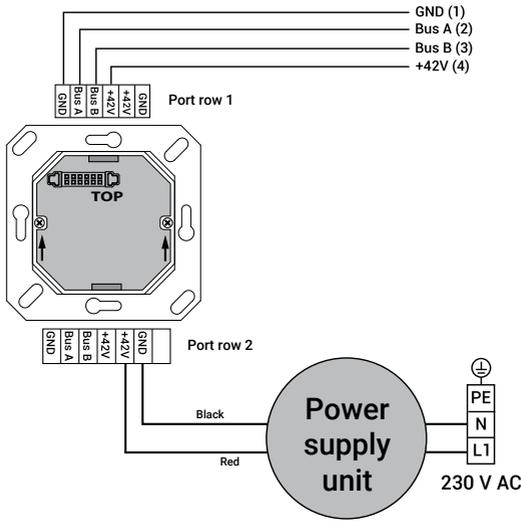
When connecting the control unit to the SmartFan unit, a 4-pin 3.50 mm connector plug must be mounted on the cable. The connector must be wired as shown below. When connecting the plug to the fan unit holder, the screws should point downwards. When continuing the cable to a further SmartFan unit, the colours of the input and output wires in the selected plug openings must match each other.
