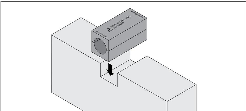
Insert the pre-fabricated Neopor® installation block into the wall, following the instructions for its installation. The hole must point downwards to the outside. Cut of any protruding material so that the block is flush with the wall.
